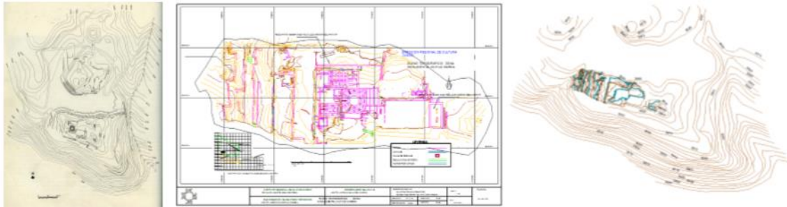
Figure 2: From left-to-right is the Historic Topographic map, the detailed AutoCad map, and the combined contour lines in GIS.
